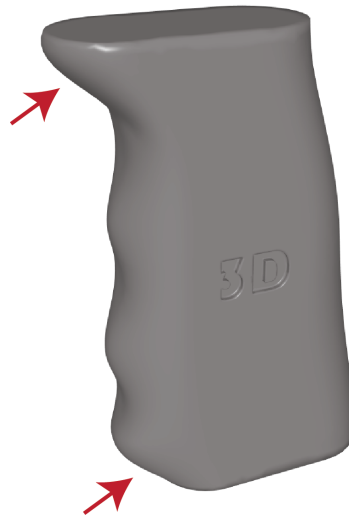
Fig. 12: An unsatisfactory deformation produced if the designer assigns too much rigidity to the finger grooves. Note the abrupt, local fluctuation of the contour of the front side, as indicated by the red arrows.
