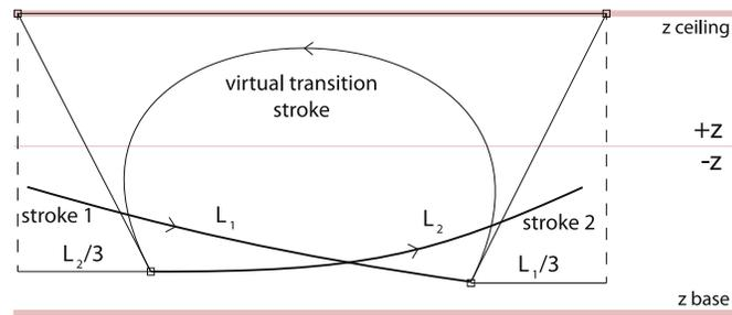
**Fig. 7.** The virtual transition strokes connect consecutive strokes. The strokes attain  $z$  coordinates based on the underlying intensities. The virtual transition strokes ascend into  $+z$  space, though not exceeding  $z_{\text{ceiling}}$ . The follow through of the transition strokes parallel to the virtual paper is determined by the underlying stroke's length.
