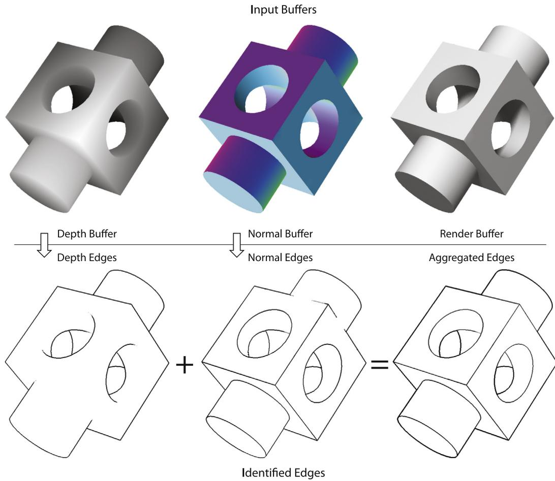
**Fig. 3.** The input buffers: depth, normal, and render buffers. The silhouettes calculated from the depth buffer and the sharp edges identified from the normal buffer are combined to identify the silhouettes and edges. The render buffer is later used for hatching.
