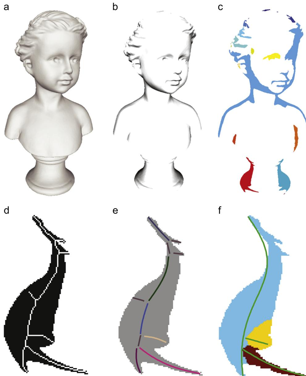
**Fig. 5.** Identification of hatching regions. (a) The render buffer is processed to determine (b) the hatching regions and shading tones (c) resulting in islands of regions. (d) For each region, the skeleton is calculated (e) and the branches are segmented. (f) Continuous branches are merged to produce compound branches from which a reduced set of regions are determined.
