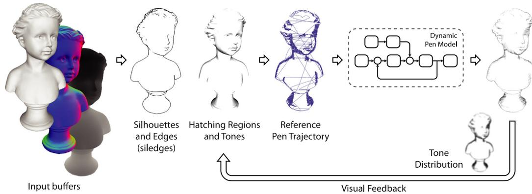
**Fig. 2.** The inputs to our system are the three render buffers. A series of silhouettes and edges are identified together with the regions to be shaded. A reference trajectory is designed for a dynamic pen model and later tracked using a closed control loop. In the outer feedback loop, the resulting render is compared to the reference render to minimize the tonal difference using hatching in multiple layers.
