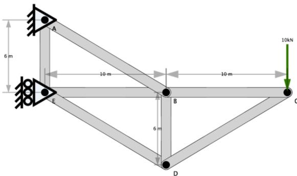
Figure 1a. Typical truss problem.
