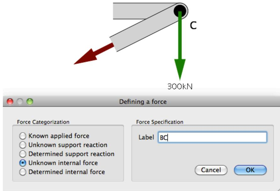
Figure 3. Screen shot of force being added to free body diagram, showing force categorization.
