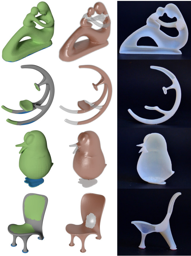
Fig. 13. Structural optimization results. Left-to-right, problem setups with fixed boundary conditions (blue) and contact regions (green), our optimized structures and 3D printed cut-outs of optimal results. Red shows the removed material.
