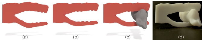
Figure 18: Initial alligator (a) is optimized (b) to hold the bunny (c). Printed and attached objects (d) exhibit the simulated/optimized behavior.
